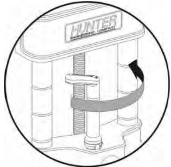
Figure 61 - To loosen, turn lever from 9 to 3 o'clock
