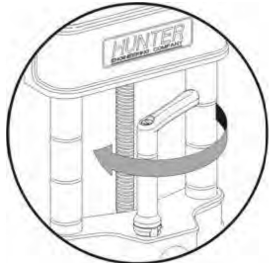
Figure 62 - To lock, turn lever from 3 to 9 o'clock
